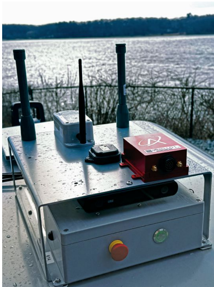
THE ANELLO MARITIME INS is equipped with three ANELLO silicon photonics optical gyroscopes for navigation in demanding maritime environments.
